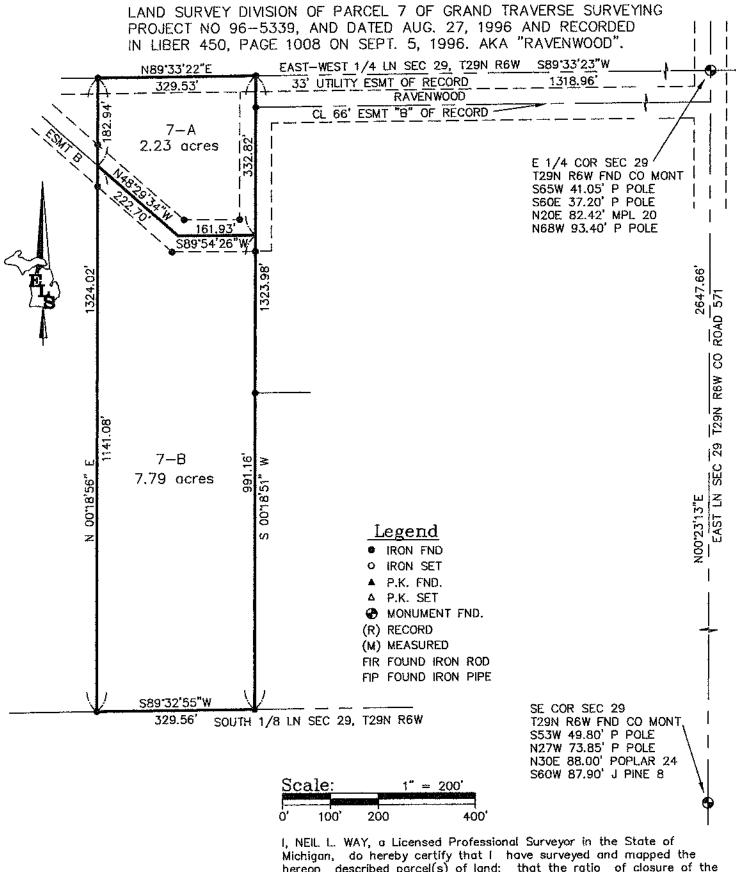
I, NEIL L. WAY, a Licensed Professional Surveyor in the State of Michigan, do hereby certify that I have surveyed and mapped the hereon described parcel(s) of land; that the ratio of closure of the unadjusted field abservations is within the accepted limits; and that I have fully complied with the requirements of P.A. 132 of 1970, as amended
